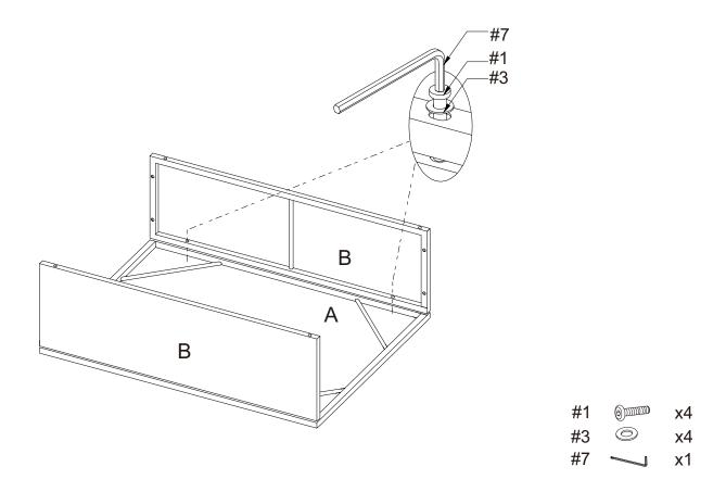
Step 2. Attach end panels (part #C) to assembled unit (parts A&B) using short bolts (part #1), washers (part #3) and allen key (part #7).
